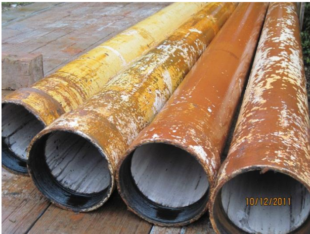
Removed column pipe-originally installed in 2004
